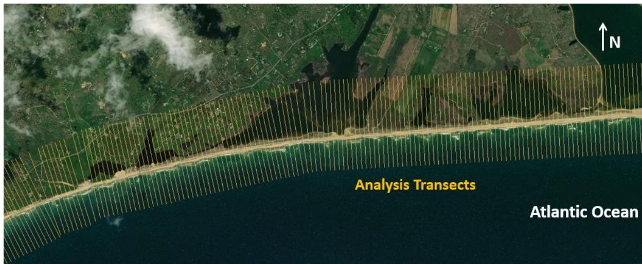
Figure 9. An example of a transect layout along a section of the FEMA Region I shoreline. For this Study, a one-dimensional (1-D) transect-based approach was implemented, where transects were placed approximately every 50 meters and oriented perpendicular to the shoreline.
