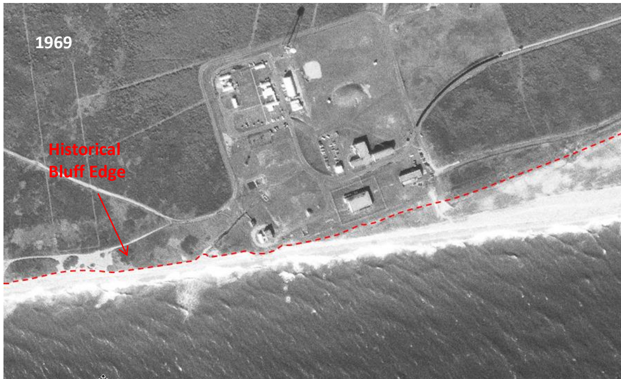
Figure 20. An example of a georeferenced historical aerial photograph from FEMA Region I. The georeferenced historical aerial photograph was used to identify the historical bluff edge (red dashed line).
