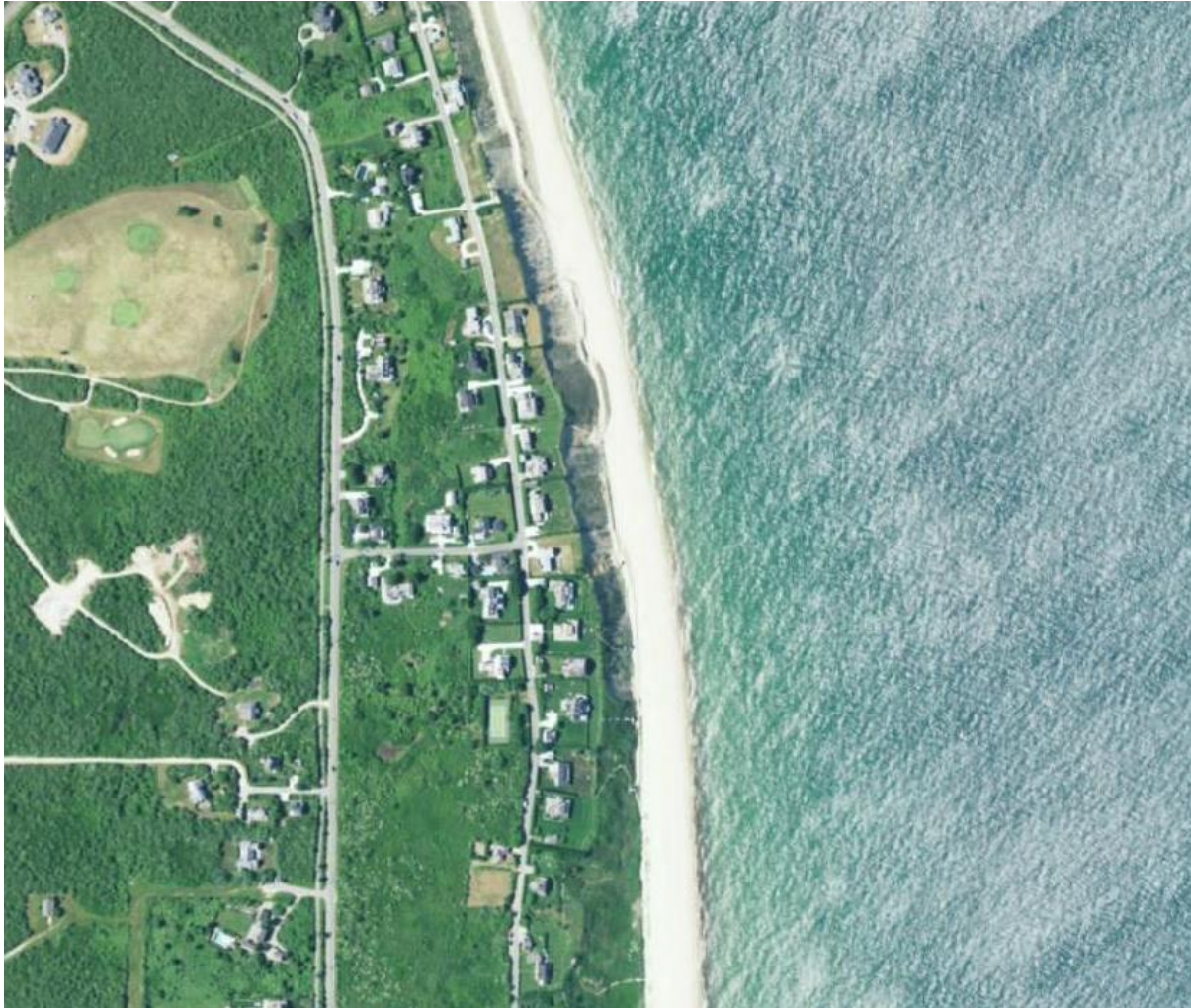
Figure 30. An example of a wide sandy beach backed by a coastal bluff from FEMA Region I. The aerial photos show that bluffs to the north are rapidly eroding. The bluffs to the south have historically been stable, although the beach is eroding. The photo shows these bluffs are well vegetated with trails and paths. Future erosion predictions for high SLR scenarios and long timeframes demonstrate that the historically stable bluffs might erode. Compass applied a hybrid analysis approach for these areas.
