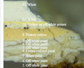
5. North elevation, fascia of cornice. Visible Light 100X
