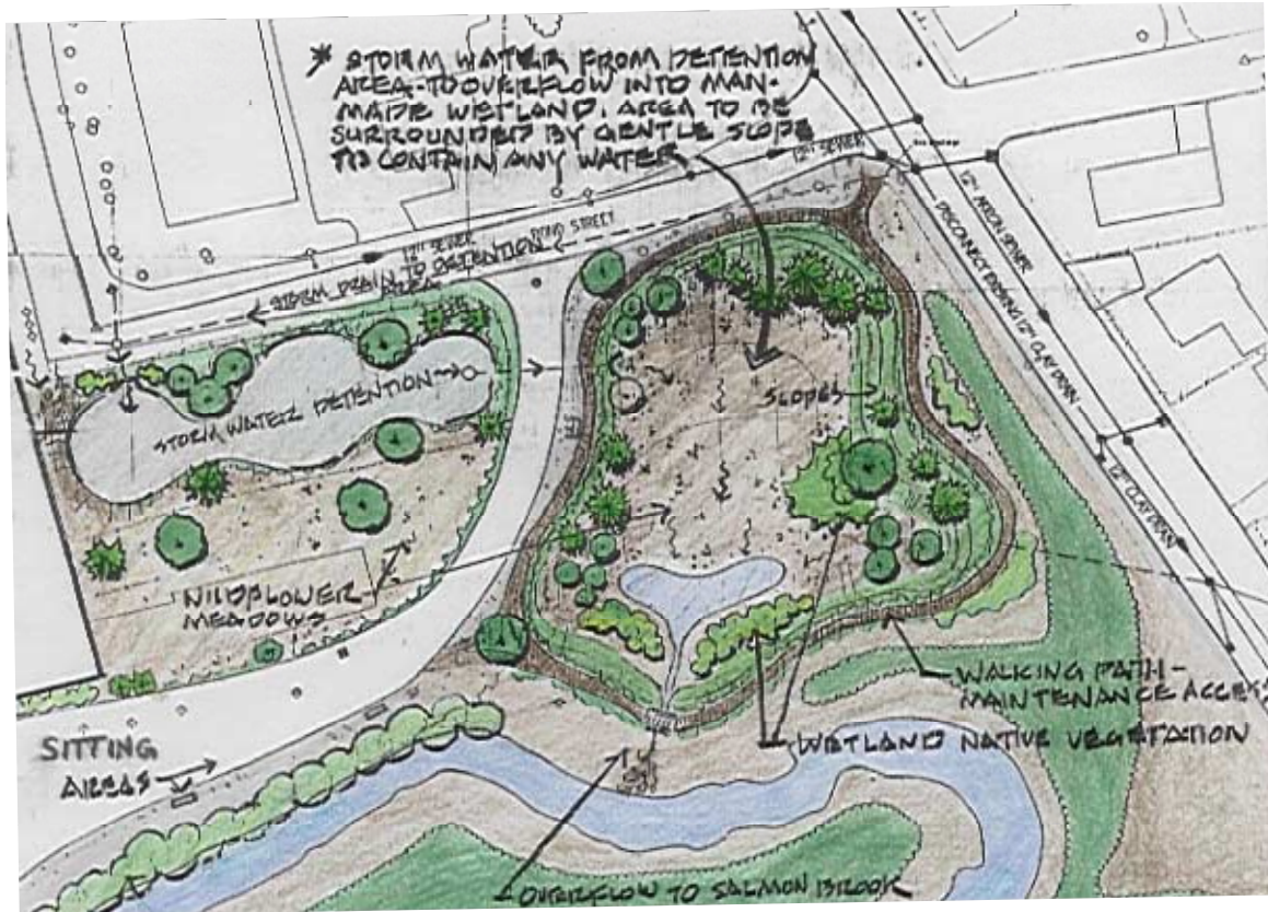
Figure 6-3. Conceptual design of wetlands treatment for roof leaders from Globe Plaza retail buildings; street runoff from Pond Street; and some separated flows from combined sewers in the area. The wetlands treatment design takes advantage of the area's high groundwater. Note that the wetlands treatment is preceded by a detention area carved out of an abandoned building rubble pile. A walking path was added to improve access to the river and sitting areas are depicted near the river bank. The access for pedestrians doubles as maintenance access for checking the overflow area and condition of the system. The design is low maintenance, with wildflower meadows near the detention basin and wetlands for treatment purposes.
